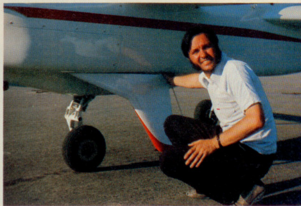
The Rutan twin cruises over 180 knots, boasts do-nothing simplicity in case of single-engine go-around. Designer Rutan points out unconventional belly-mounted rudder. Photos by the author.
