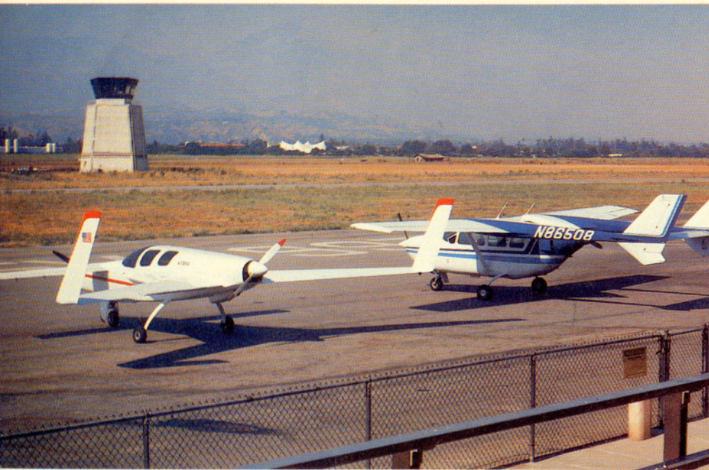
Two generations of push-pull twins share the ramp at Brackett Field, Calif. The Defiant could spur the simple-twin concept begun by the Cessna Skymaster—but will it be produced?
